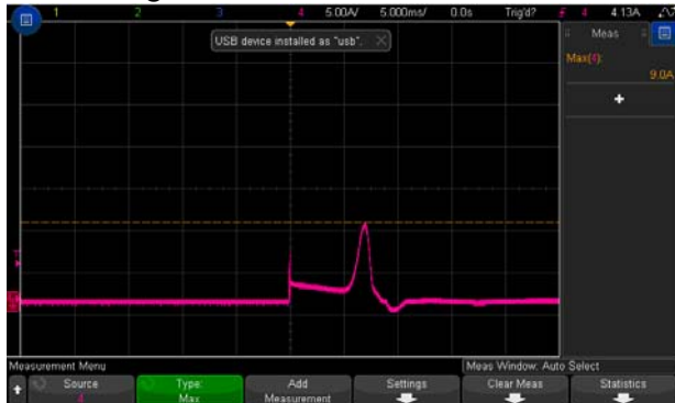
INPUT=24VDC @ FULL LOAD
